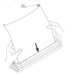
Figure 9. Inserting a sheet of paper
